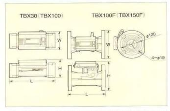
The display unit on the TBX100F (TBX150F) can be freely moved about to match the gas flow direction. In addition, the entire display unit can be removed and placed up to three meters away.
