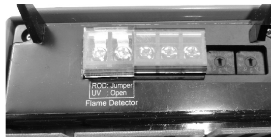
ULT Model (bus connector and address switches)
